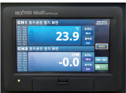
Set and control temperature and flow rate
